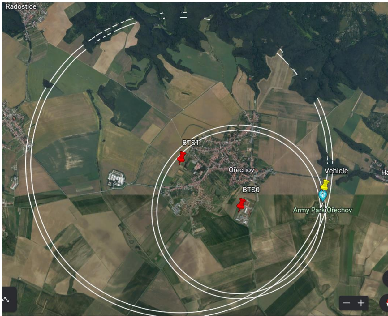
Figure 5: Blue point showing position estimate from Timing Advance, the yellow pin shows location per GPS.
