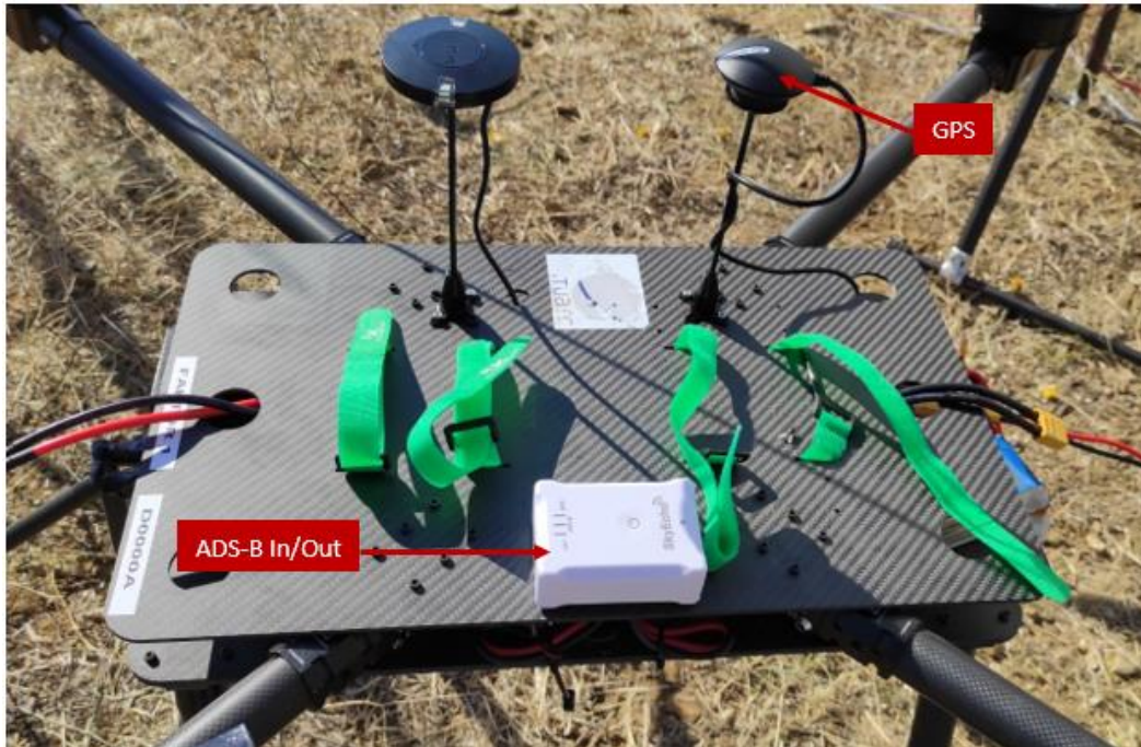
Figure 19. ADS-B In/Out uAvionix SkyEcho installed on top of the drone
