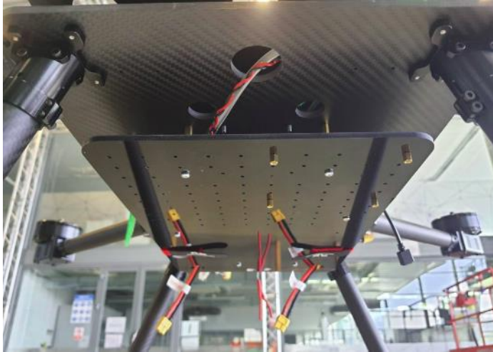
Figure 23. Carrier plates for Honeywell’s Experimental CNS device and its peripherals.
