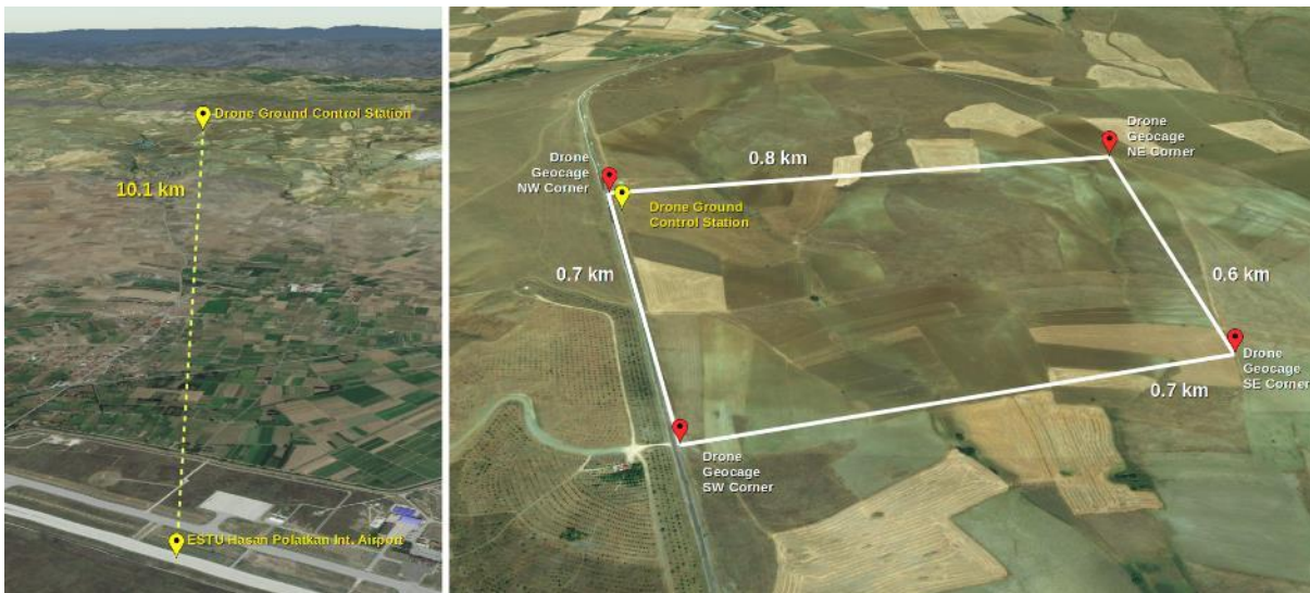
Figure 3 Ground Control Station and the Geocage
