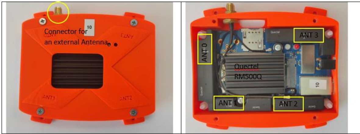
Figure 14. Housing for Quectel RM500Q – version for use of integrated antennas
