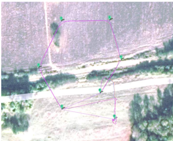
Figure 14. From waypoint 1 to 6, the drone flew in autonomous mode. Take-off and landing phases were piloted flight.
