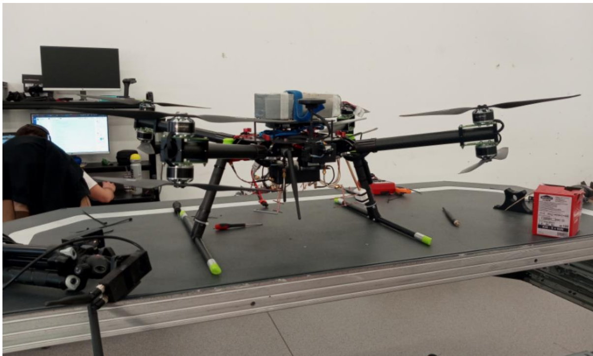
Figure 2. Experimental device mounted on drone during USpace4UAM flight trials (the black box on the drone's belly).
