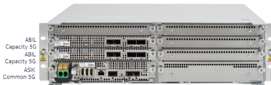
Figure 18. AirScale subrack example with one ASiK and two ABiLs
