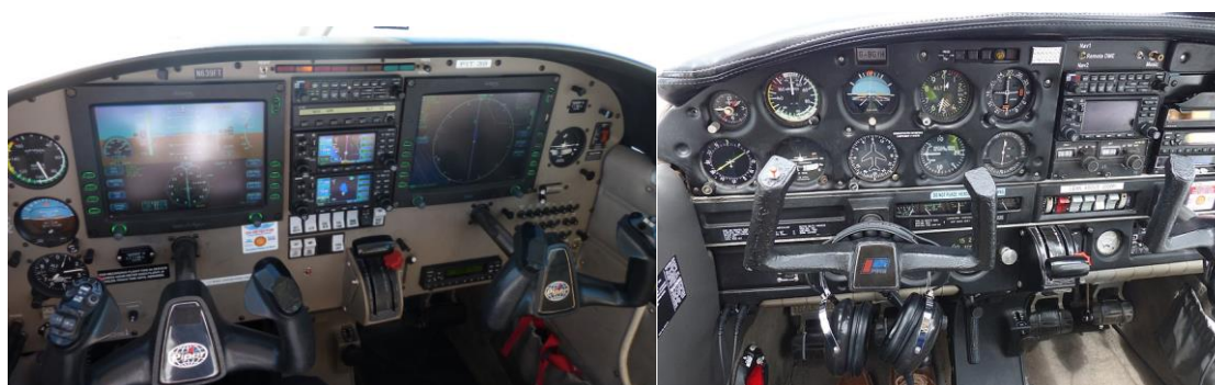
Figure 6: Piper Cherokee Cockpit with Avidyne Entegra PFD and MFD and with federated avionics
