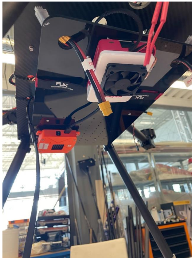
Figure 9: Experimental CNS system platform mounted under the demonstration drone.
