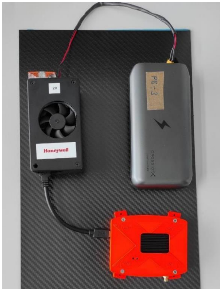
Figure 3: Experimental CNS device for installation on drone (here connected to power bank but on drone it uses power from drone).
