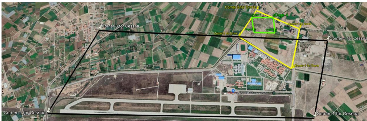
Figure 20: Scenario 1 airspace configuration (black = GA flight, yellow = drones' allocated area, green = planned geocage area).
